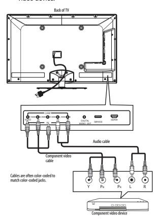
3 Connect an audio cable to the AV/COMP L/R audio jacks on the back of your TV and to the L/R AUDIO OUT jacks on the component video device.
